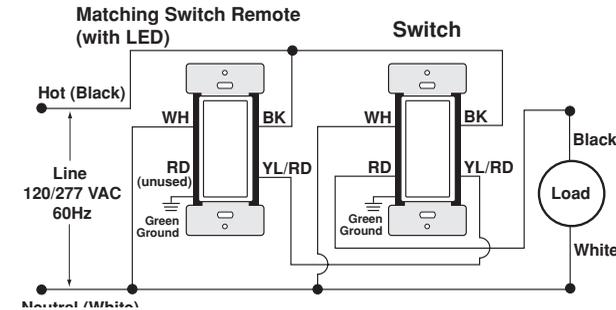
**NOTE:** The switch **must** be installed in a wall box that has a Load connection. The matching remote must be installed in a wall box with a Line Hot connection and a Neutral connection. A Neutral wire to the matching remote needs to be connected as shown.
