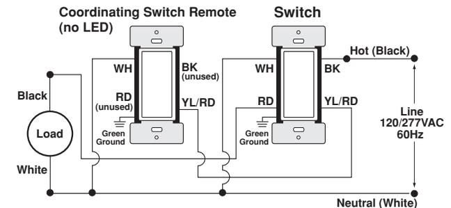
**NOTE:** The switch must be installed in a wall box that has a Line Hot connection. The coordinating remote must be installed in a wall box with a Load connection and a Neutral connection. A Neutral wire to the coordinating remote needs to be added as shown. If you are unsure about any part of these instructions, consult an electrician.
