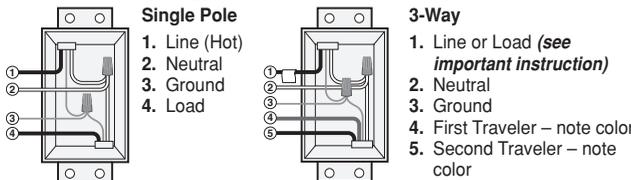
**IMPORTANT :** For 3-Way applications, note that one of the screw terminals from the old switch being removed will usually be a different color (Black) or labeled Common. Tag that wire with electrical tape and identify as the common (Line or Load) in both the switch wall box and remote wall box.
